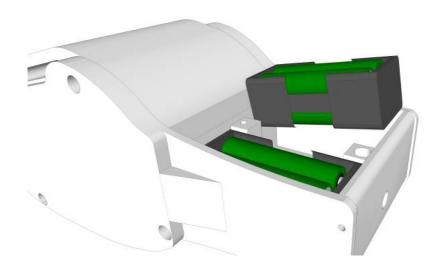
Replace the batteries. Watch the polarity and make sure to use the <u>same battery type</u> and that they are all new. Lithium AAA batteries are the best! Push the holders back in.
