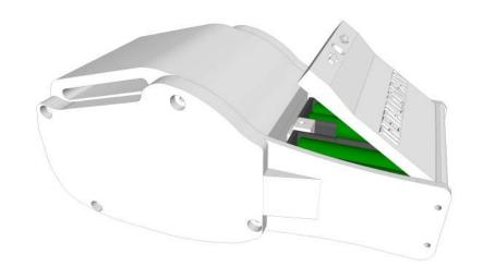
Lift out the battery holders gently, but be careful not to damage the wires!
